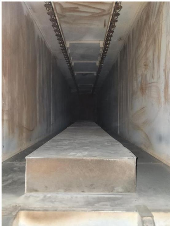
Hot Air Convection Drying (LNG Burner)
