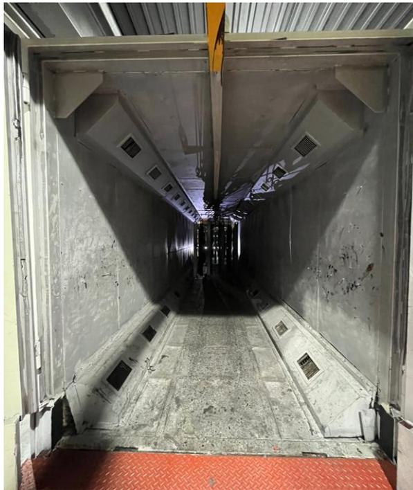
Hot Air Convection Drying (LNG Burner)
